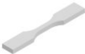
Tensile ASTM D638 - Type V
