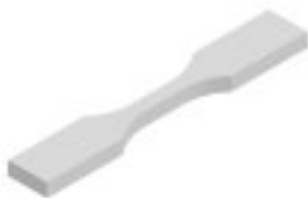
Tensile ASTM D638 - Type V
