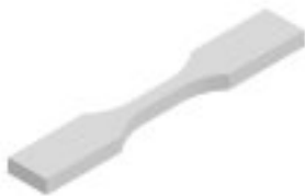
Tensile ASTM D638 - Type V
